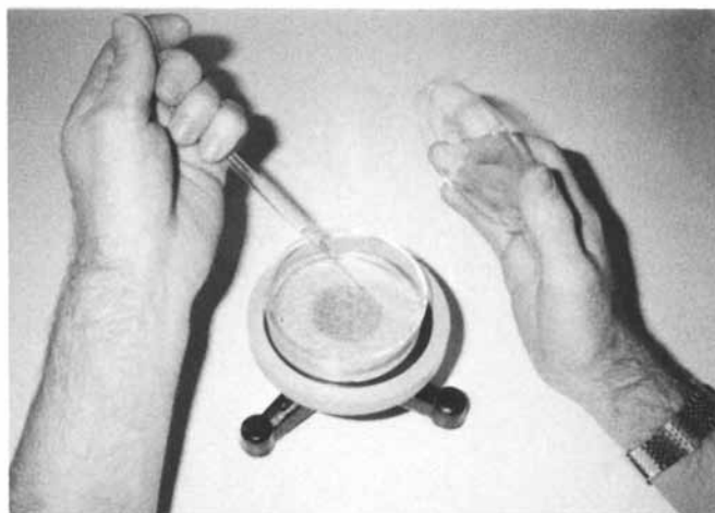
Figure 2. Illustration of the technique used to distribute high numbers of A. thaliana seed onto petri plates.
